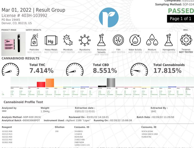
Full spectrum cannabinoid analysis utilizing High Performance Liquid Chromatography with DAD detection (HPLC-UV). Method SOP-022 (R13) for reporting. Lower limit of linearity for all cannabinoids is 1 mg/L.
